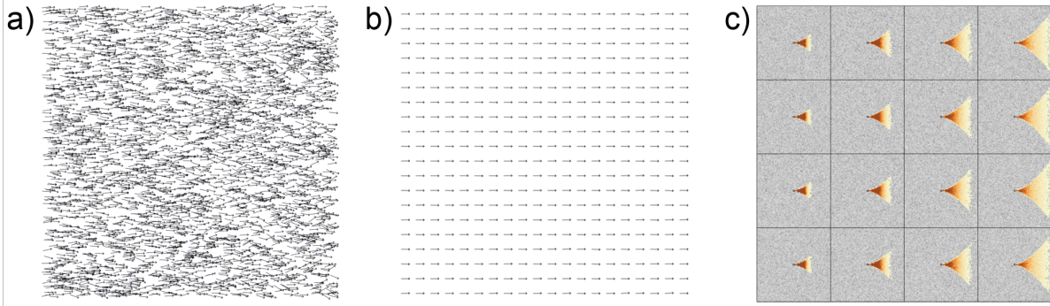
Figure 3: A synthetic particle dataset designed to show the advantages of using the histogram based representation. a) Attaching a velocity vector to each particle results in a great deal of clutter. b) Averaging particle velocities into a vector field eliminates important flow patterns. c) The histogram based view provides a low clutter decomposition of the velocities in each part of the domain.
