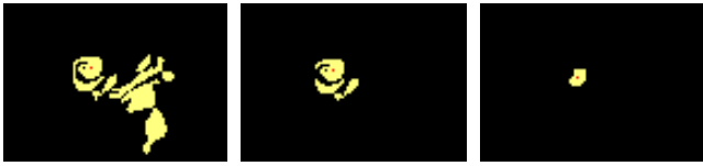
Figure 3. 2D slice of different shapes extracted from a constant seed point (red) by adjusting the threshold value; the images from left to right represent an increasing threshold.
